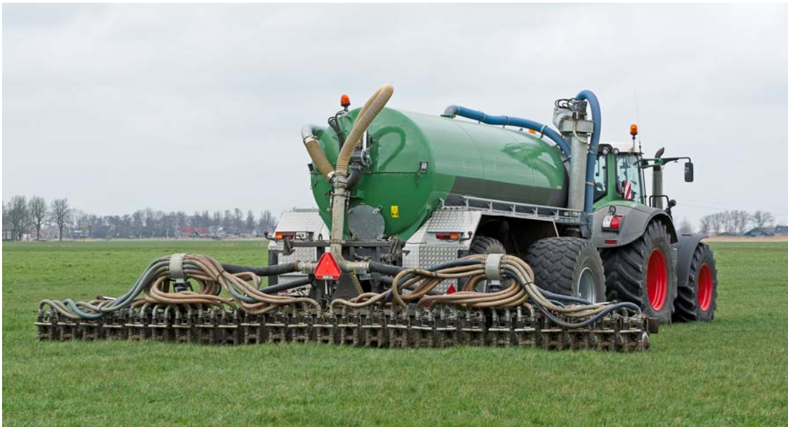
A tractor injects liquid biosolids into the soil.
