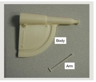
2. Paste the clinometer label on to the body of clinometer with the glue stick. Place the label so that the edge of the "0" line is flat against the raised ridge and the round cut-out portion at the top of the label is flush against the hole (see image below). This ensures that the measurements are accurate.
